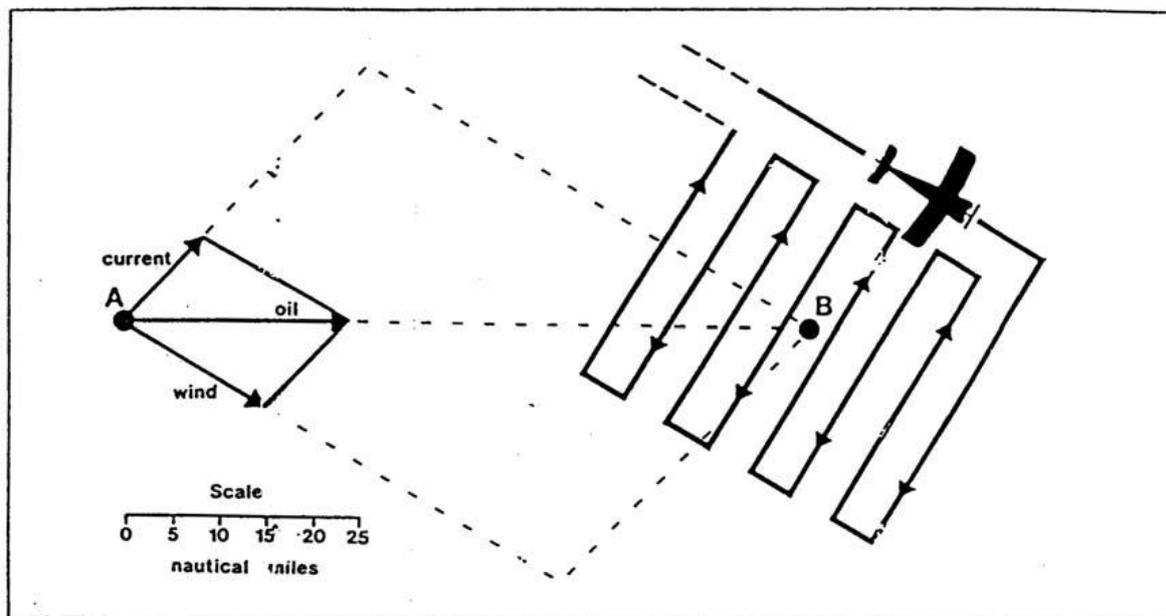
Movement of oil from A to position B three days later, predicted by combining 100% of the current speed and 3% of the wind speed as shown. The arrows from A represent current, wind and oil movement for one day. A cross-wind ladder search pattern is shown over position B.
