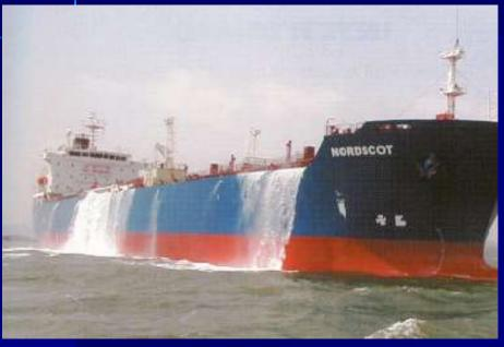
at least three times per volumetric capacity of each ballast tank discharge/pumping • water exchange must involve at least 95% of the ballast water volume "flow through"
