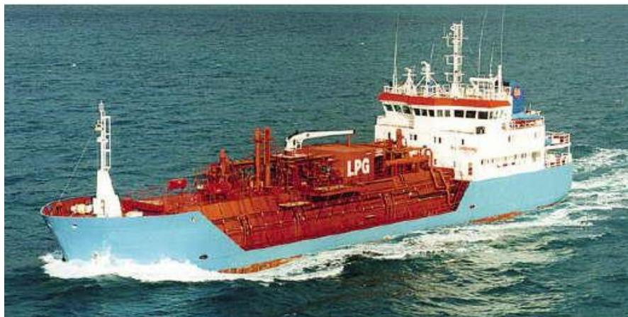
**Figure 9.** *An example of a semi-pressurized LPG/NH<sub>3</sub> carrier*
