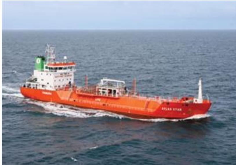
**Figure 11.** An example of a semi-pressurized/fully refrigerated ethylene/LPG carrier
