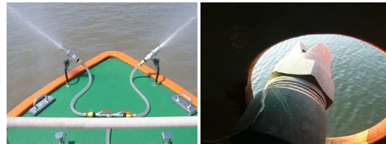
Figure 28. a) mobile single-nozzle cannon (© Clean Caribbean & Americas), b) fixed system integrated directly into the ship's hull (© TotalEnergies).
