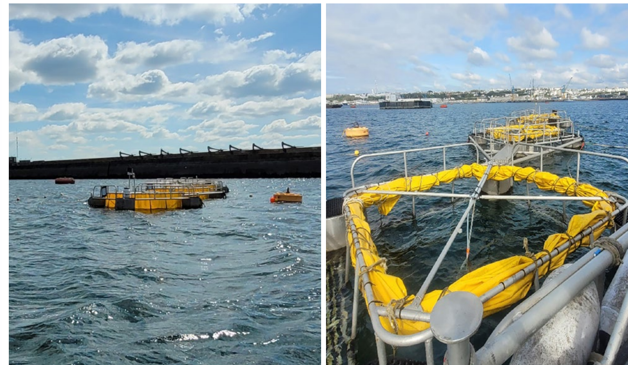
Figure 11. Floating cells used by Cedre for test under in situ conditions (@Cedre). Objective : conduct tests under natural conditions.
