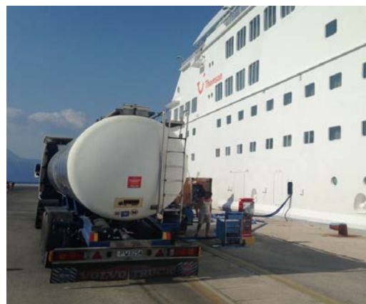
Tank truck collecting liquid waste from a cruise ship (Photo credits: Peter Van den dries)
