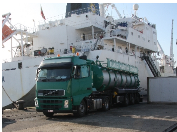
Tank truck collecting oily waste (Photo credits: Kayak Maritime Services, Antwerp, Belgium)
