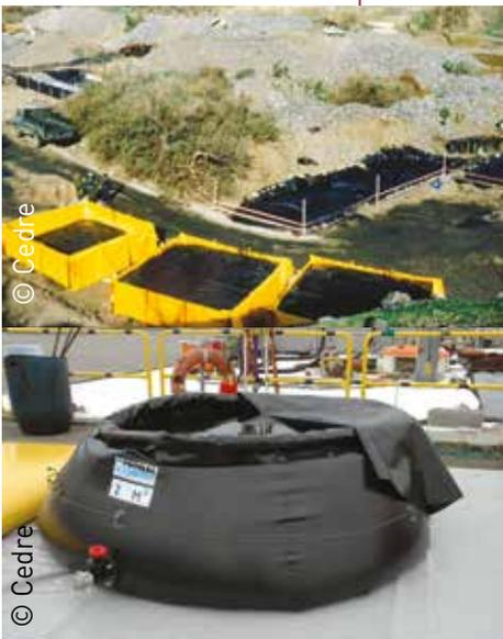
Large open top collapsible container with supporting frame (5 to 140 m<sup>3</sup>)
