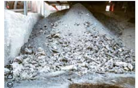
Ash and clinker remaining after burning and to be disposed of
