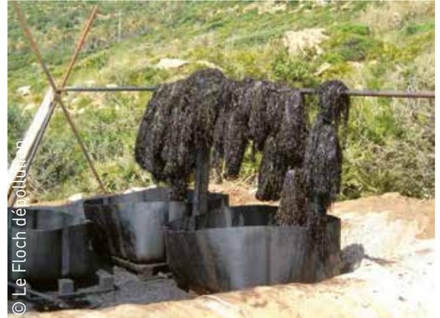
■ ■ Example of recycling used PPE as sorbent for oil collection on water surface
