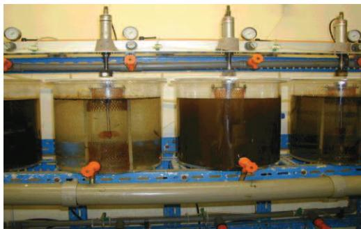
**Figure 10: Toxicity tests with shrimps conducted on dispersed oil in UK**
