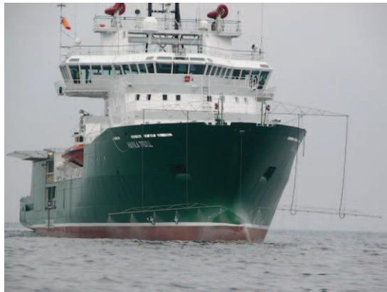
**Figure 20: Ship mounted modern application spraying equipment (source SINTEF)**
