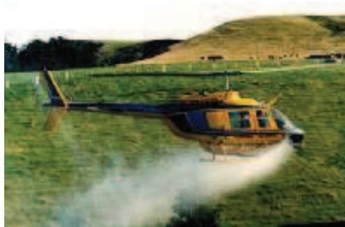
**Figure 25: Fixed spraying systems for helicopter**
