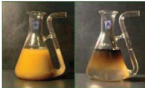
**Figure 17: The swirling flask test method (source: [www.marinemanagement.org.uk/protecting/pollution/documents/approval\\_lr448.pdf](http://www.marinemanagement.org.uk/protecting/pollution/documents/approval_lr448.pdf))**
