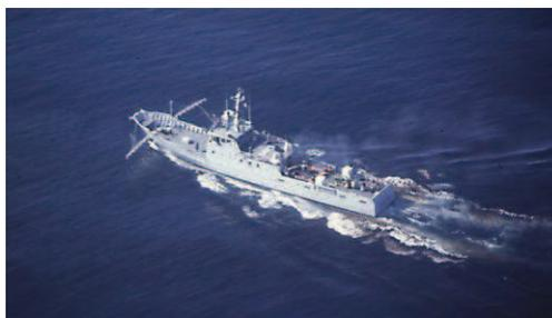
**Figure 8: Ship applying dispersant
