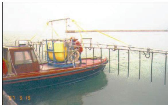
**Figure 27: Conventional dispersant spraying system for boat**
