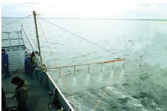
**Figure 28: Application of dispersant pre-diluted into sea water**
