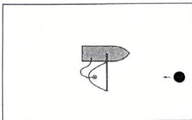
Single vessel system: boom and recovery device deployed from one vessel, generally with the help of a jib.
