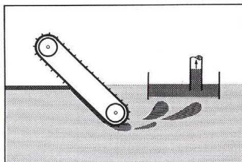
**Figure 6** Operating principle of conveyor belt skimmer
