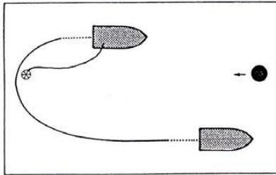
J - configuration: boom towed by two vessels and recovery unit deployed from one of them.
