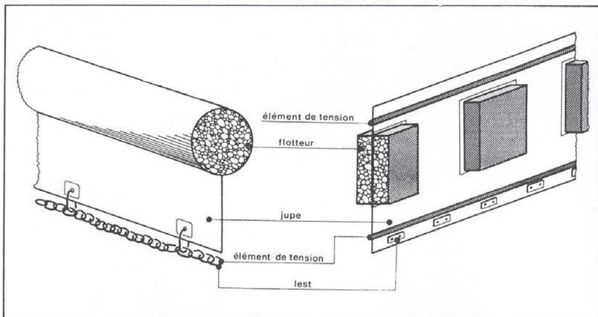
**Flotation element** (float) provides for the buoyancy of the whole system (boom), but often functions as an additional freeboard to reduce splash-over. It can be filled either with some solid material (expanded plastic foams e.g. polyethylene, polyurethane, polystyrene or natural flotation materials e.g. cork, wood, etc ...) or with air.
