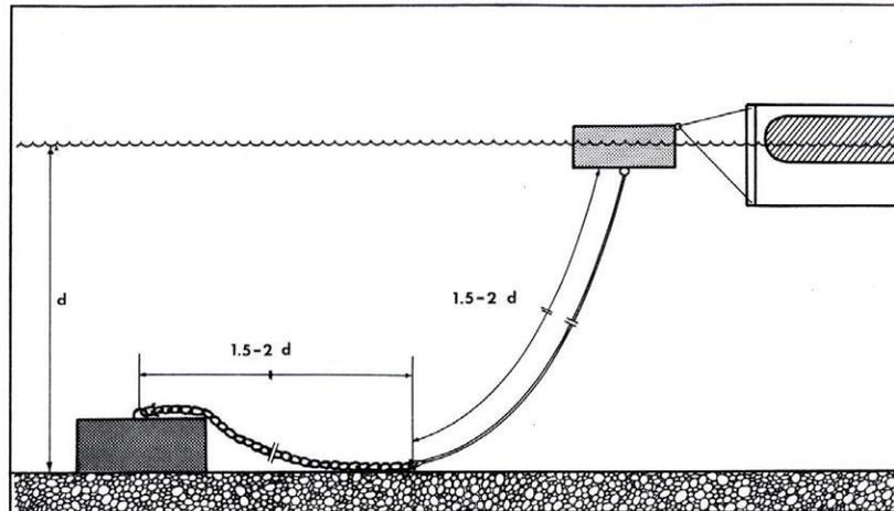
If an end of the boom (or both) is to be anchored to a shoreline, it can either be attached to an existing object (large tree or man-made structure) or an anchor system should be constructed. Very good results are obtained by so called "deadman". It is a log or beam buried in the hole in the direction perpendicular to the maximum pulling force expected:
