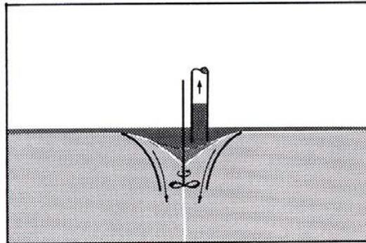
**Figure 4** Operating principle of dynamic vortex type skimmer
