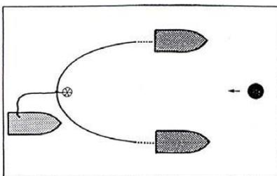
U - configuration: boom towed by two vessels and recovery unit deployed from a third one.
