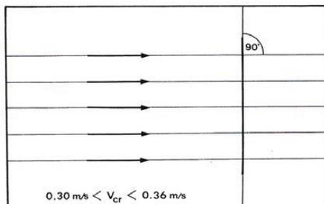
It was discovered that if the current velocity at right angles to a boom's section exceeds a certain value, oil starts escaping underneath the boom. For most of the booms this "critical velocity" is between 0.58 and 0.70 knots (0.30 and 0.36 m/s).
