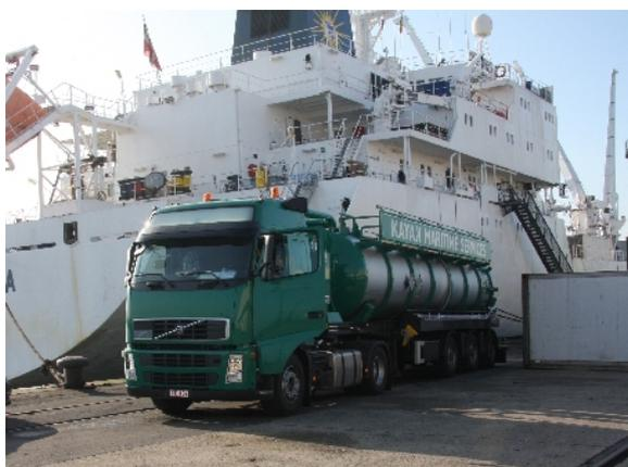
Tank truck collecting oily waste
