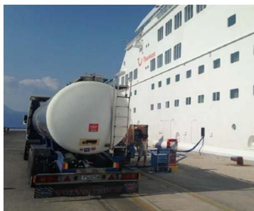
Tank truck collecting liquid waste from a cruise ship
