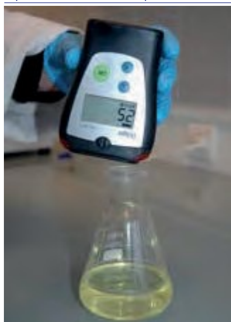
Vapour measurement with an explosimeter.
