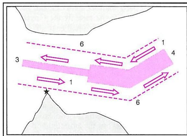
Figure 2 – Traffic separation by separation zone.
