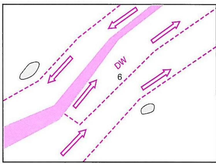
Figure 4 – One-way deep-water route (within a traffic lane)
