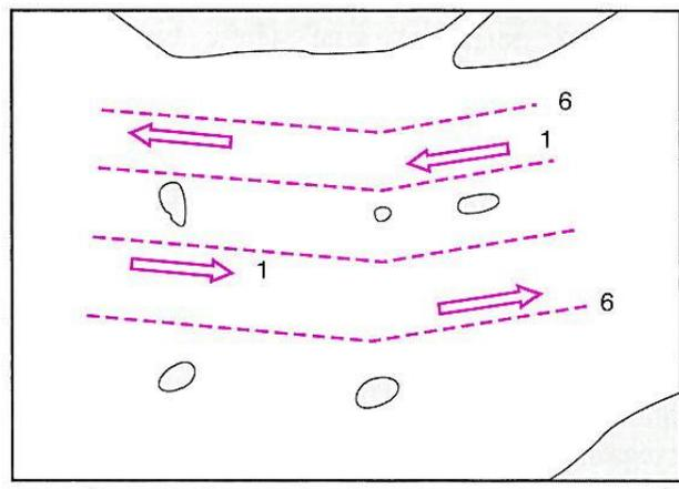
Figure 3 – Separation of traffic by natural objects
