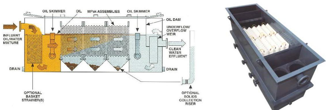
API separators, described in section 3.3.1, can be retrofitted with plate packs to increase the separation efficiency.
