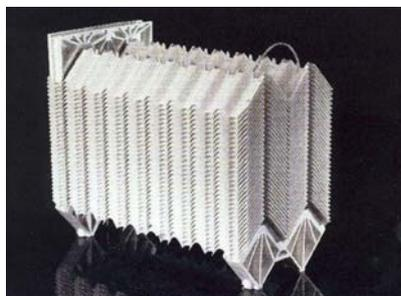
The use of a coalescing plate separator is appropriate for oily water streams with relatively low particulate impurities. The units are able to handle low to medium flow ranges. For larger flow rates, a modular design is applied i.e. several smaller units operate in parallel.
