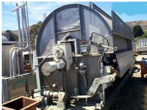
A vacuum filter consists of a hollow cylinder covered with a filtering medium made of cloth, plastic or stainless steel. As the cylinder revolves, a vacuum is applied to a section of the drum immersed in the wet sludge. By increasing the vacuum, water is drawn through the filtering medium, leaving the sludge in the form of a cake that is discharged after one revolution.
