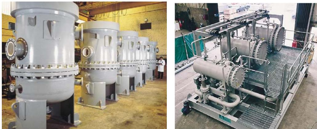
The efficiency of hydro cyclones is poor in viscous fluids with constituents of relatively low specific mass differences. Hydro cyclones are commonly applied in the oil industry (on- and offshore) for separation of solids or oil from water. The units shown in the pictures above contain a number of hydro cyclones in each vessel, to increase the treatment capacity and/or separation efficiency.
