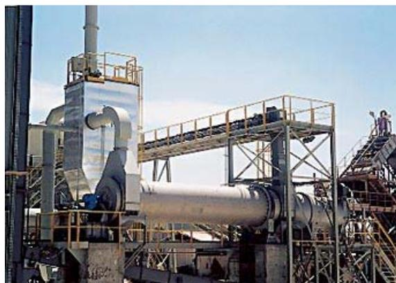
The standard dryer sizes are based on evaporation rate capacities of one or several metric tons per hour. Drying results in a volume reduction of the waste to be disposed of, but has no other benefits.
