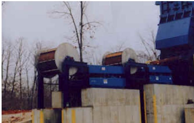
The Self-Cleaning Recycling Magnets are Permanent Magnets using the latest and highest grade of materials suitable for this type system. When compared to electro magnets, no electrical source is required for the magnet, it is considerably lighter in weight, has a lower profile, is virtually maintenance free and less expensive to purchase, install and operate.
