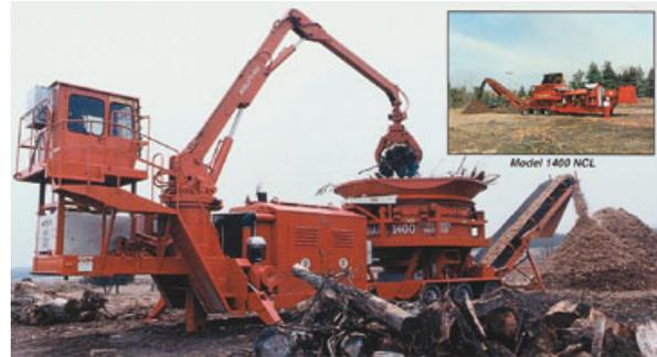
The equipment can be operated by one operator and uses a high speed grinding design to quickly reduce waste (drive engine power 1.5kW - 300kW)..
