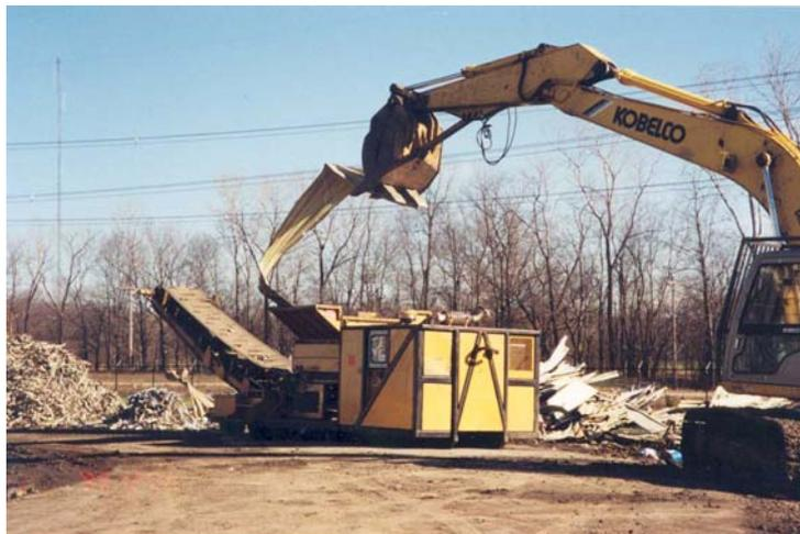
There are different designs possible like single shaft, high torque, low speed shear shredders for size reduction of baled materials or twin shaft, high torque, low speed shear shredders for size reduction of general waste (electrical motor power 15kW - 320kW).
