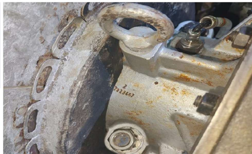
A turbocharger with IMO ID number as per the Technical File.
