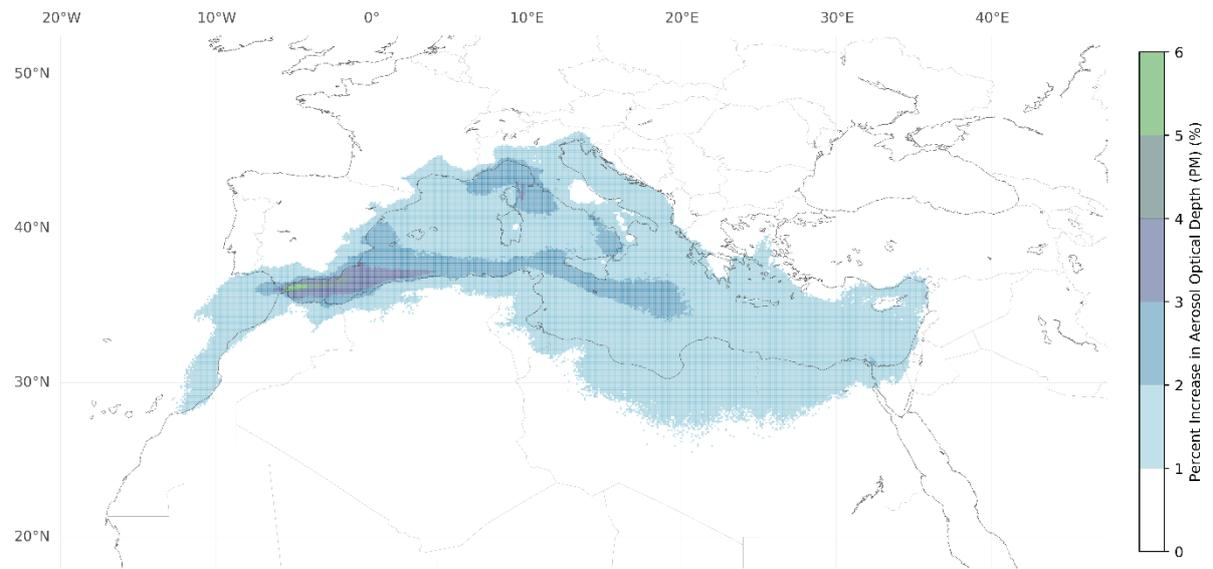
Figure 25. Percent Change in aerosol optical depth (PM species) between MARPOL VI and the proposed Med ECA
