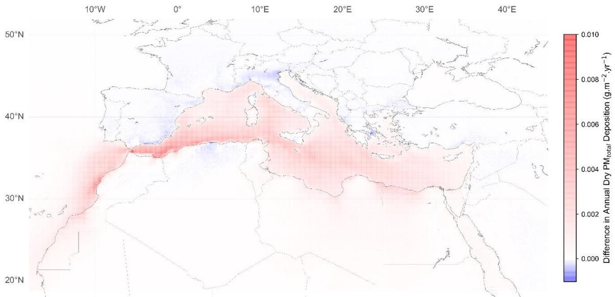
Figure 23. Change in annual dry  $PM_{Total}$  deposition between MARPOL VI and the proposed Med ECA
