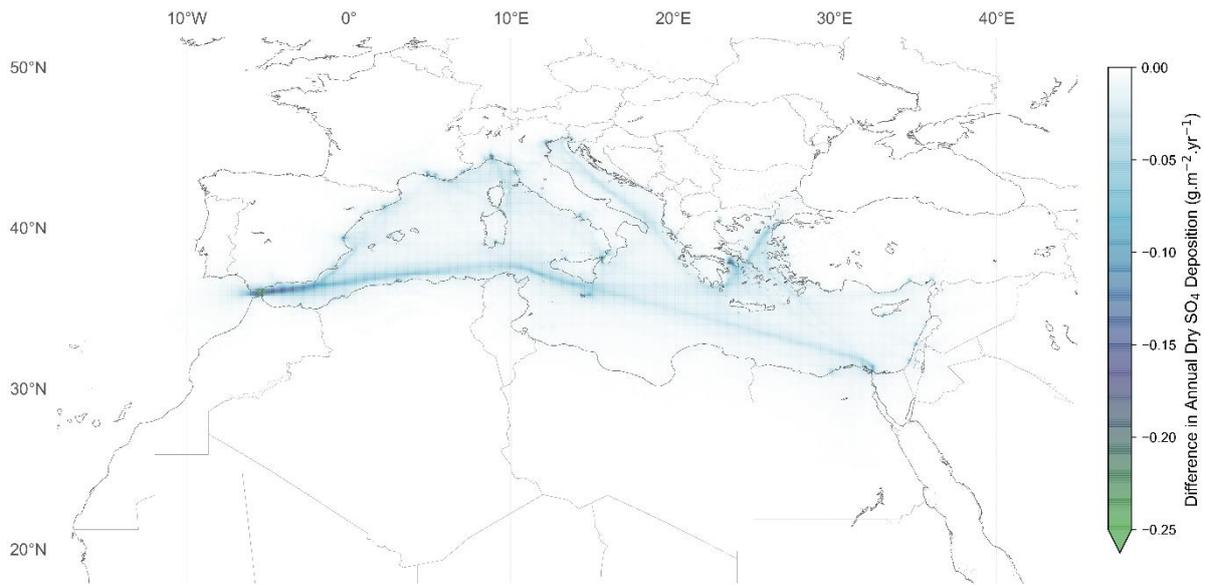
Figure 19. Decrease in annual dry sulphate deposition between MARPOL VI and the proposed Med ECA
