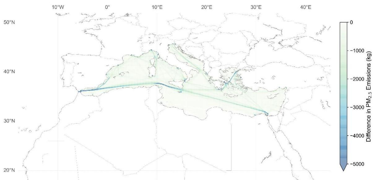
Figure 11. Geographic distribution of reduction in PM<sub>2.5</sub> emissions (in kg) between MARPOL VI 2020 fuels (0.5% S) and proposed Med ECA 2020 fuels (0.1% S)
