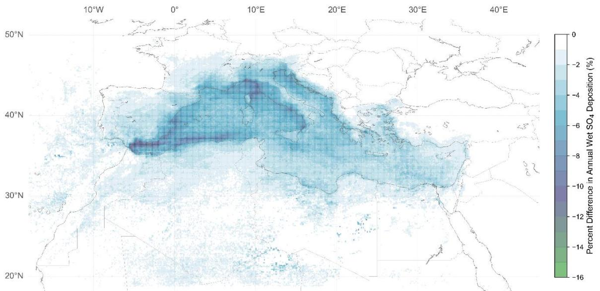
Figure 18. Percent decrease in annual wet sulphate deposition between MARPOL VI and the proposed Med ECA
