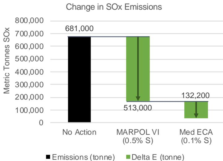
Figure 12. STEAM modeled reduction in total SO<sub>x</sub> emissions in the Mediterranean Sea from 2016 baseline, to MARPOL VI (0.5% S) and the proposed Med ECA (0.1% S) scenarios
