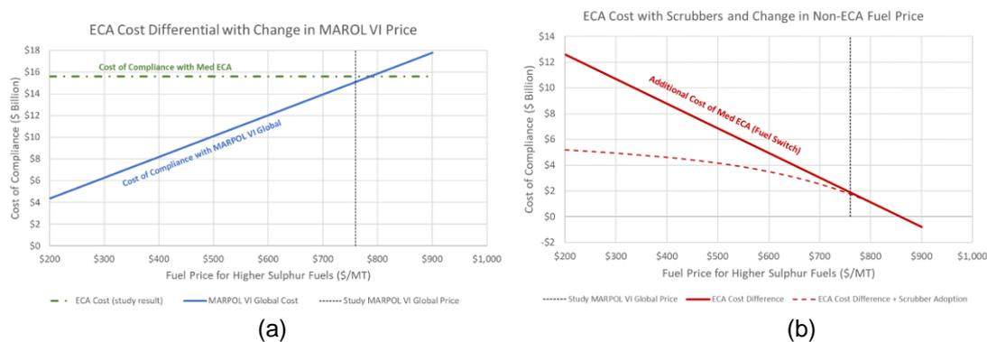
Figure 28. Summary graphs of SECA cost sensitivity to fuel price for non-SECA (higher-sulphur) fuels, and scrubber adoption: (a) cost difference between switching from MARPOL VI global fuel to SECA fuel; and (b) additional cost to comply with the proposed Med ECA including potential economically feasible adoption of scrubber technology
