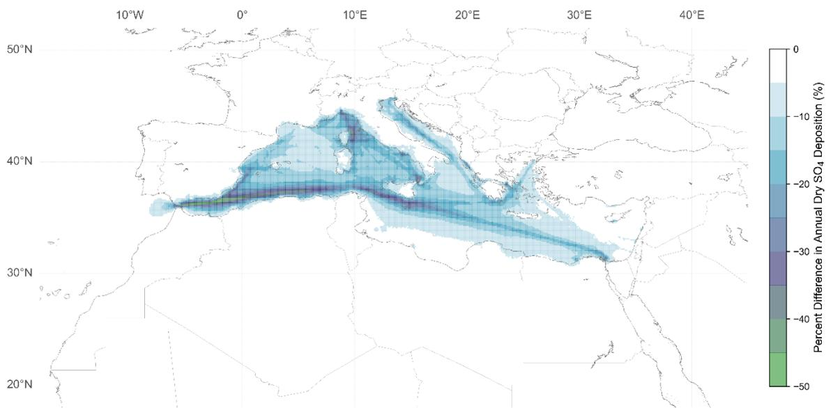
Figure 20. Percent decrease in annual dry sulphate deposition between MARPOL VI and the proposed Med ECA
