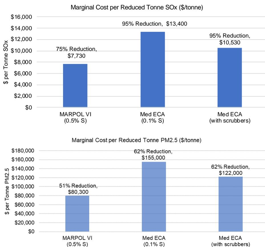
Figure 29. Control cost-effectiveness of SO<sub>x</sub> and PM<sub>2.5</sub> reductions based on prices in this study
