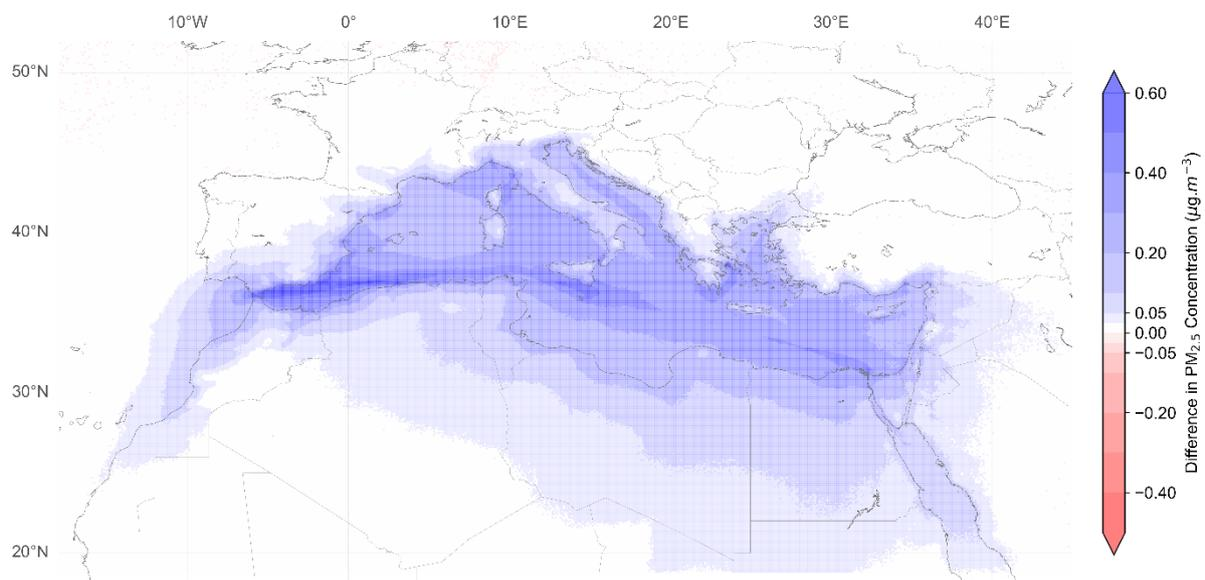
Figure 16. Difference in PM<sub>2.5</sub> concentration between MARPOL VI and the proposed Med ECA scenarios
