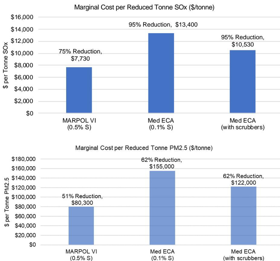
Figure 5. Control cost-effectiveness of SO<sub>x</sub> and PM<sub>2.5</sub> reductions based on prices in this study
