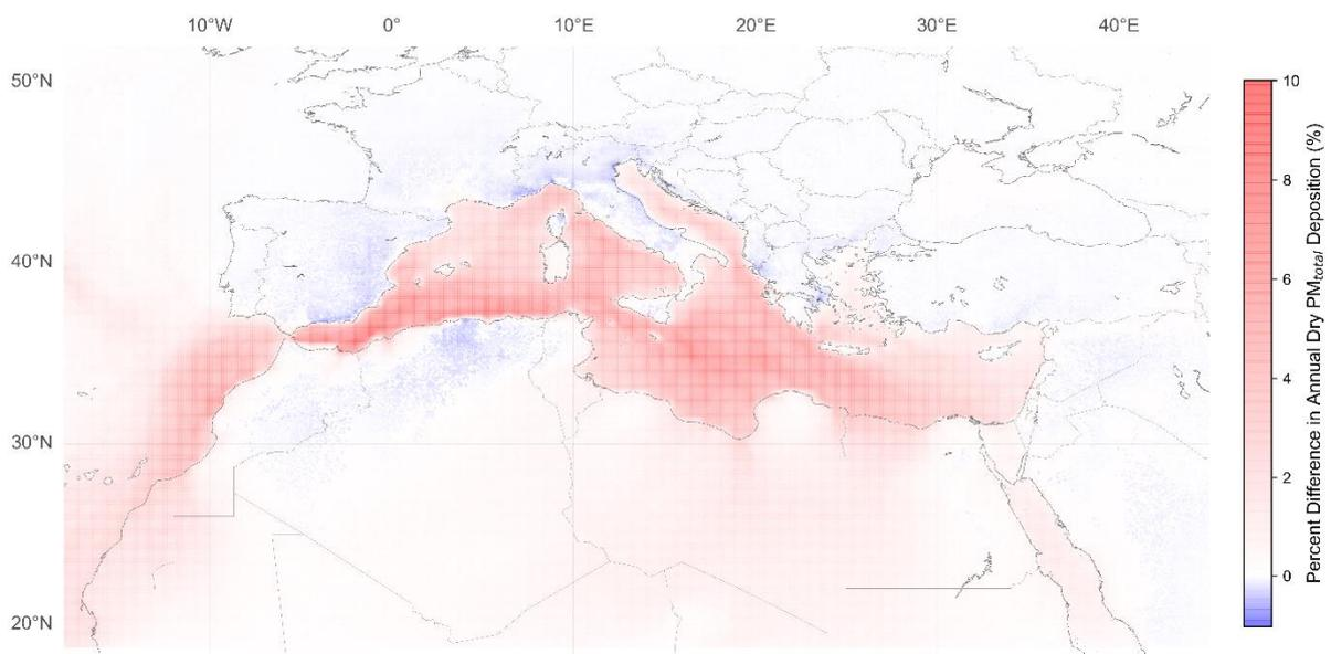
Figure 24. Percent change in annual dry  $PM_{Total}$  deposition between MARPOL VI and the proposed Med ECA
