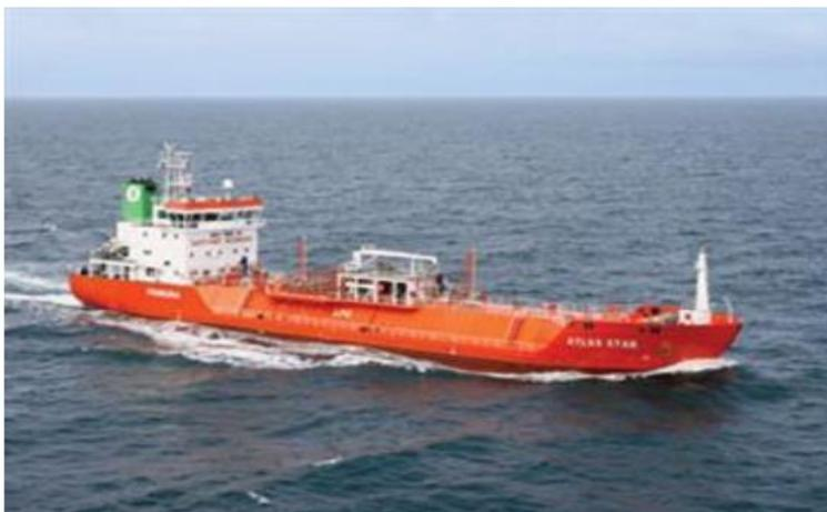
**Figure 18.** An example of a semi-pressurized/fully refrigerated ethylene/LPG carrier.
