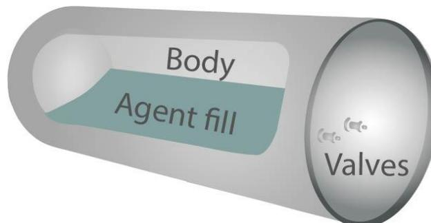
***Figure 10 (Copyright Cedre). Example of a ton container.***
