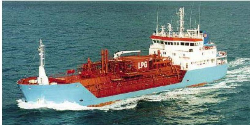
***Figure 16. An example of a semi-pressurized LPG/NH<sub>3</sub> carrier.***
