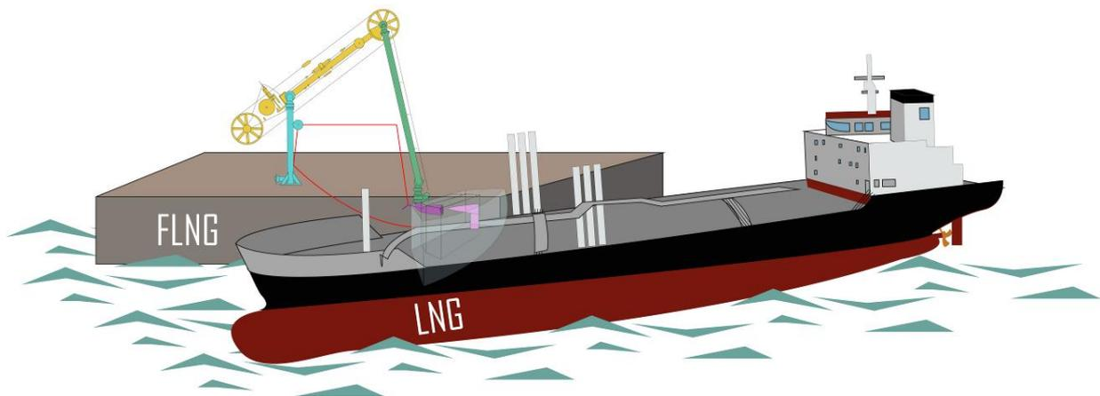
**Figure 24. Side-by-side LNG offloading system.**
