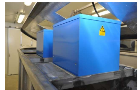
UV units simulate solar radiation
